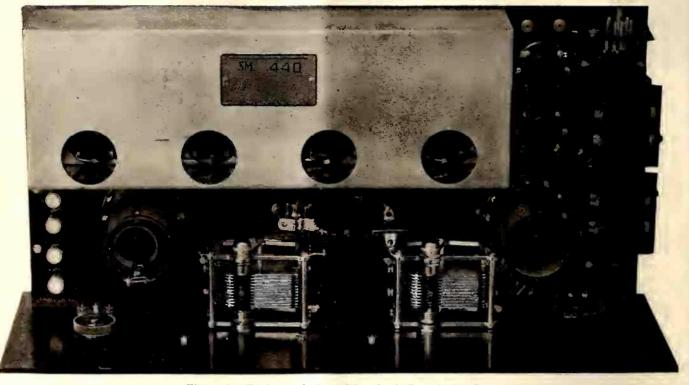
Figure 1.—Back panel view of Quadrode Superheterodyne
